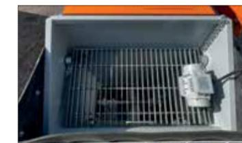
PC 158 is a 2-cylinder hydraulic piston pump with S-valve and variable output for pumping concrete, micro-concrete, special concrete and for shotcrete.
