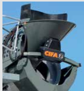
Rubber sleeve on the loading hopper.
