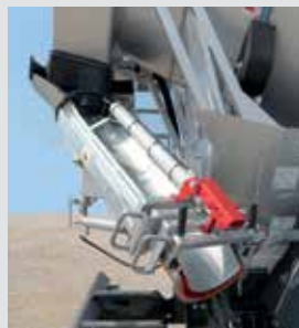
"SL 45" hydraulic extractable discharge chute.
