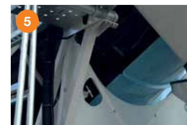
Drum safety stop for truck mixer maintenance and plastic back cover.
