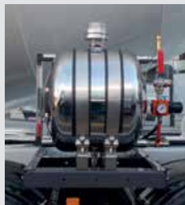
Additive pressurized tank (50 l) made of stainless steel
