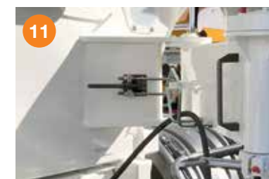
Mono-support arm for discharge chute (for SL and SLX series).
