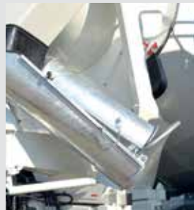
Fold over chute (1500 mm + 600 mm).
