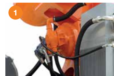
Water pump installed on the reducer.
