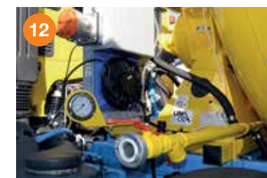
Double water inlets. Water can be filled from both right and left side of the truck mixer. Heat exchanger with oil tank. Manometer for concrete consistency.
