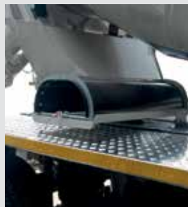
Special supports for chutes placed at 90° underneath the drum.
