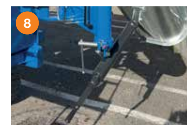
Chute lifting by crank handle.
