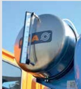
Aluminum pressurized water tank (capacity from 200 to 800 liters).
