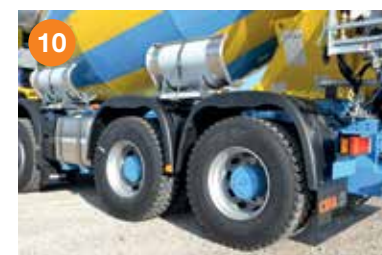
Polymer rear mono-axle mudguards. Double-axle mudguards made of aluminum are available on demand.
