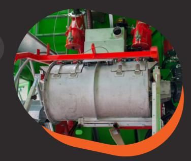
This innovative OVERMAT equipment is made up of a pre-mixer, in which the raw materials selected in the formula are conveyed and dosed, and two pumping tanks that are easily interchangeable on the jobsite: one mixer vessel is dedicated to the pressure pumping of conventional dry screed and the other one to the pumping of liquid screed with screw pump.
